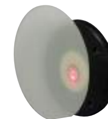
With a transparent Sapphire sample the two DiP beams can be observed.
