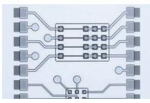
For spacing out chip dies in fan-out packaging applications, they are bonded onto wafers or panels after dicing. The bonding process introduces small position shifts, which become a limiting factor as the density of wiring traces increases. The MLA 300 can expose unique patterns for each substrate, taking into account the die shift, so that traces are exposed in their intended place.
