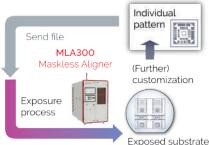
The benefit of Maskless Lithography is the inherent rapid turnaround and adaptation of the exposed patterns. Modifications for customized products no longer entail production and maintenance of an expensive mask set. Switching between product types is seamless, and does not require intervention to change masks.
